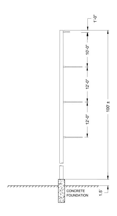
> STEEL HORIZONTAL POST TYPICAL 138kV STRUCTURE
