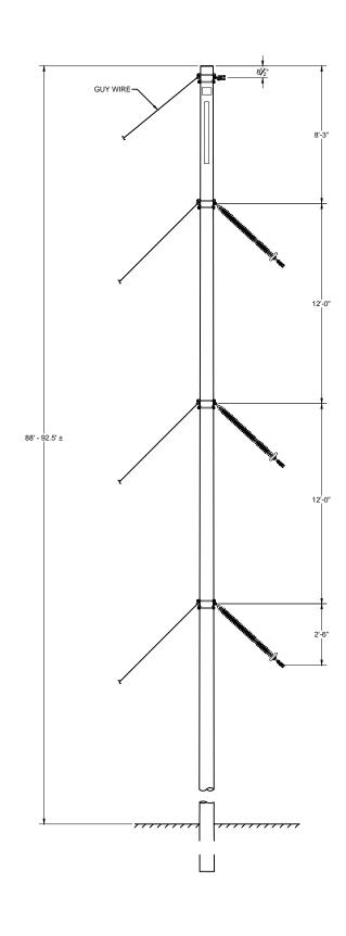
WOOD SUSPENSION VERTICAL TYPICAL 138kV STRUCTURE
