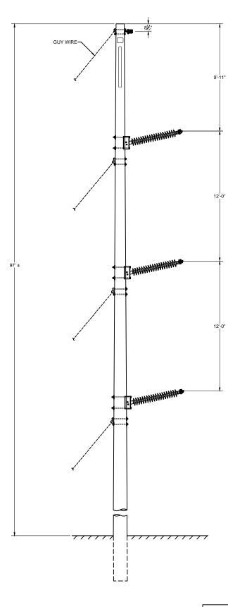
WOOD HORIZONTAL POST VERTICAL TYPICAL 138kV STRUCTURE
